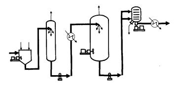
For the continuous bleaching of edible fats and oils • Excellent color reduction and soap removal • Low clay dosage. Low oil retention • Effective deaeration and dehydration. Effective oil-clay contact • Efficient utility usage. Minimum operator attention • Automatic control of process variables.
